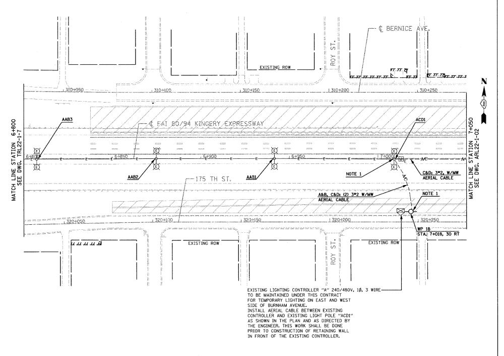
NOTE 1. SEE DETAIL AT DRAWING NO. ADL22-01 FOR TEMPORARY AERIAL CABLE CONNECTION TO EXISTING LIGHT POLE.
