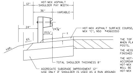
t = SEE TYPICAL SECTIONS FOR THICKNESS
