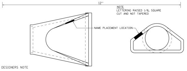
NAME PLATES SHALL BE FURNISHED & INSTALLED ACCORDING TO SECTION 515 OF THE STANDARD SPECIFICATIONS, EXCECT 2 BOLTS SHALL BE USE TO FASTEN THE PLATE TO THE END SECTION.
