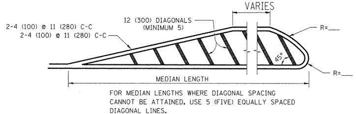
DIAGONAL LINE SPACING: 50' (15 m) C-C (LESS THAN 30MPH (50 km/h)) 75' (25 m) C-C 30MPH (50 km/h) TO 45MPH (70 km/h)) 150' (45 m) C-C (MORE THAN 45MPH (70 km/h))
