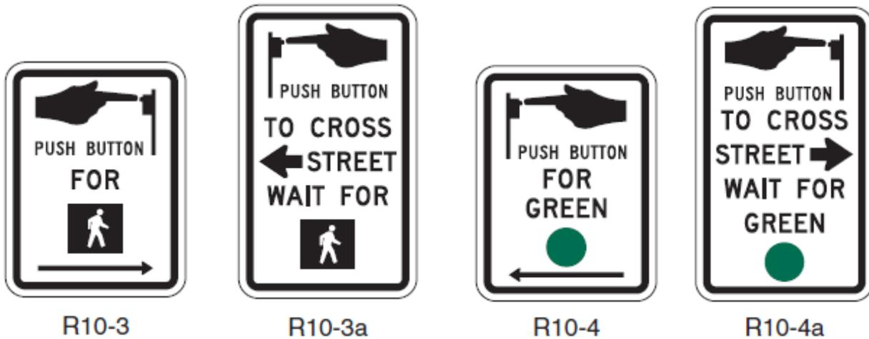
Tactile Arrow. A tactile arrow, pointing in the direction of travel controlled by a pushbutton, shall be provided either on the pushbutton or its sign.
