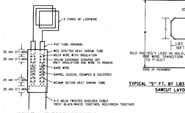
EDGE OF PAVEMENT TYPICAL "S" FT. BY 1.83 m (6FT.) INDUCTION LOOP SAWCUT LAYOUT FOR RAMPS
