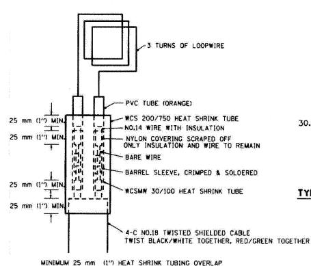
ON WIRE, PVC & SHIELDED CABLE TO FORM WATER TIGHT SEAL
