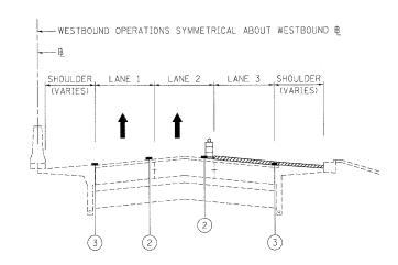
STAGE III - OPERATION FOUR - I-290 BITUMINOUS SURFACE REMOVAL FINAL, 2" - LANES 3, 4 & 5 BITUMINOUS SURFACE REMOVAL FINAL,  $1-\frac{3}{4}$  - AUXILLARY LANE, SHOULDER, & INSIDE OF ROOSEVELT ROAD RAMPS TO I-88
