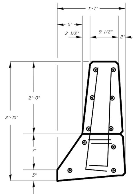
**TYPICAL PARAPET SECTION**
