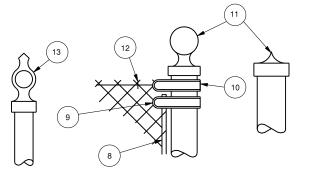
POST TOPS TO BE PRESSURE FITTED OR SCREWED. POST TOPS MAY BE ELIMINATED FOR ALL POSTS EXCEPT PIPE POSTS. IF POST TOPS ARE ELIMINATED, POST LENGTH
