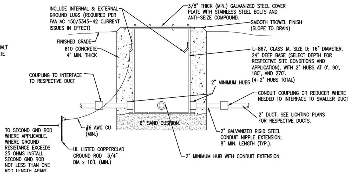
**SPlice CAN/JUNCTION CAN DETAIL**
