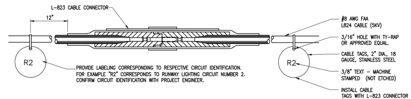
1. CONTRACTOR SHALL PROVIDE CABLE CIRCUIT IDENTIFICATION MARKERS ATTACHED TO BOTH SIDES OF EACH CABLE CONNECTION.
