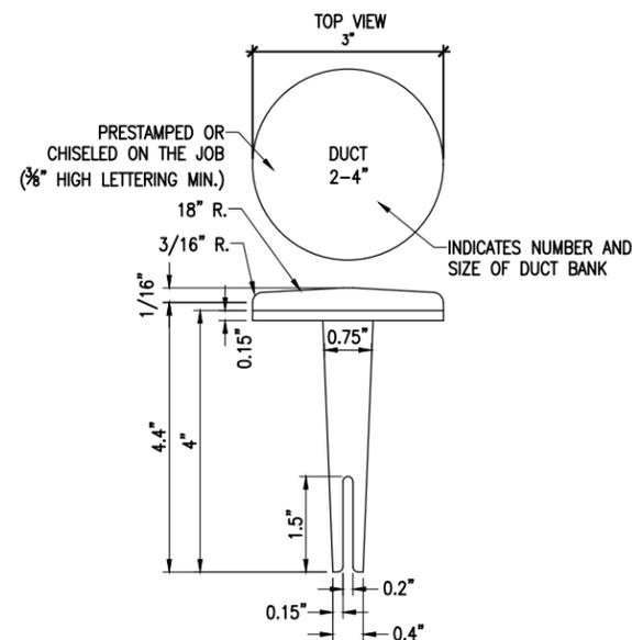
BITUMINOUS PAVEMENT DUCT MARKERS
