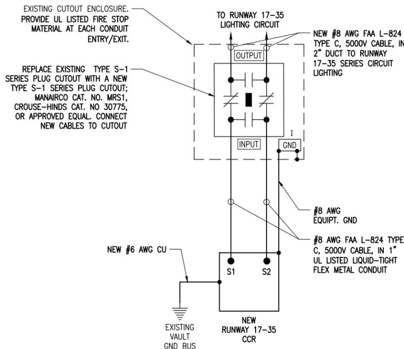
**PROPOSED HIGH VOLTAGE WIRING SCHEMATIC FOR RWY 17-35 CCR**
