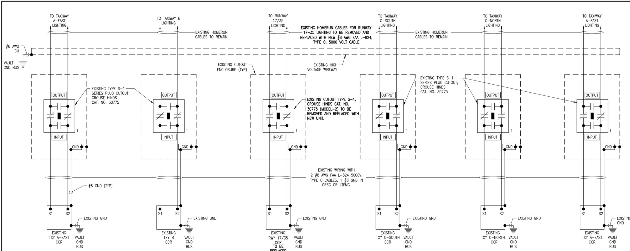
**EXISTING HIGH VOLTAGE WIRING SCHEMATIC FOR RUNWAY 17-35 & TAXIWAYS**
