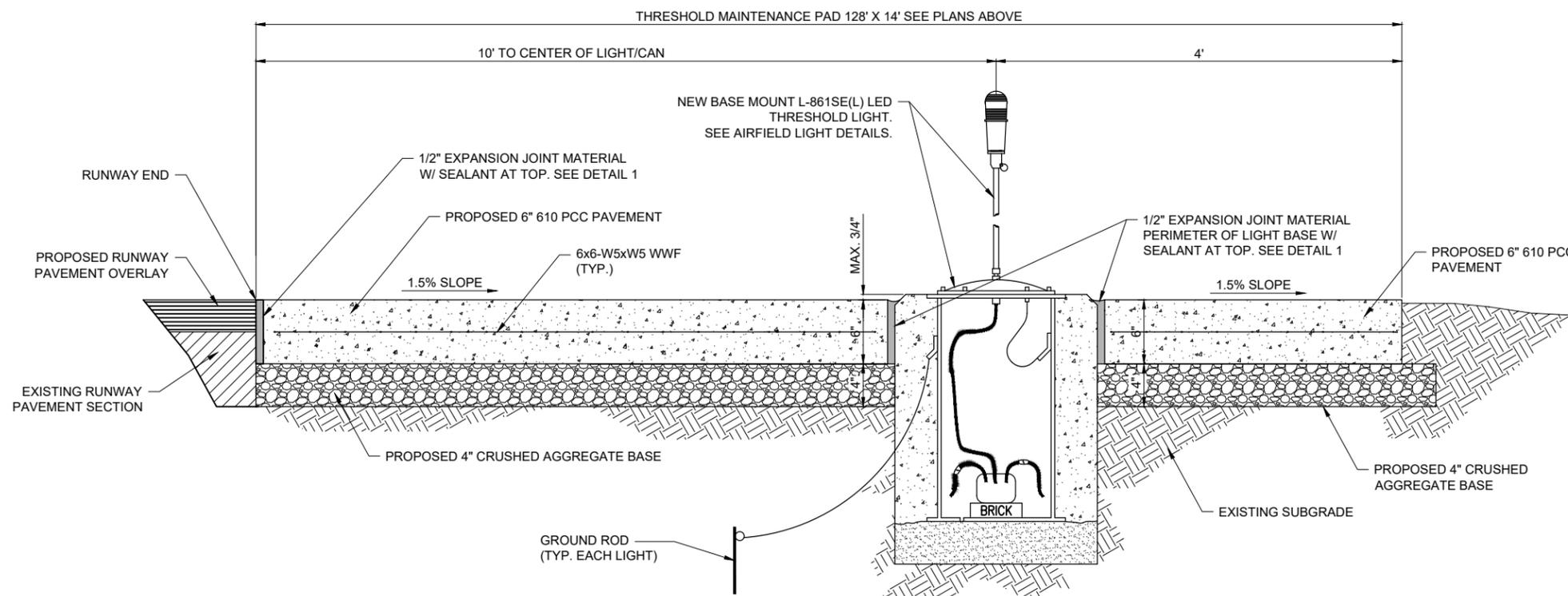
THRESHOLD LIGHTING MAINTENANCE PAD DETAIL
