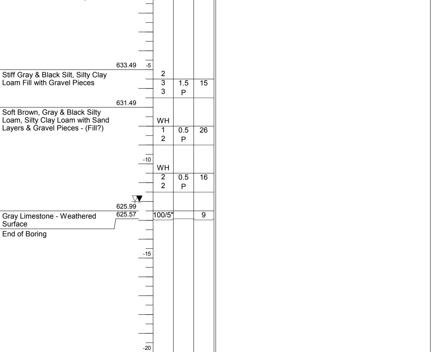
The Unconfined Compressive Strength (UCS) Failure Mode is indicated by (B-Bulge, S-Shear, P-Penetrometer)
