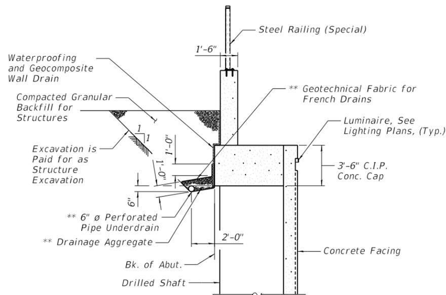
**SECTION THRU TOP OF WALL BETWEEN ABUTMENTS**
