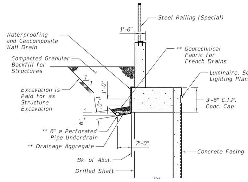
SECTION THRU TOP OF WALL BETWEEN ABUTMENTS
