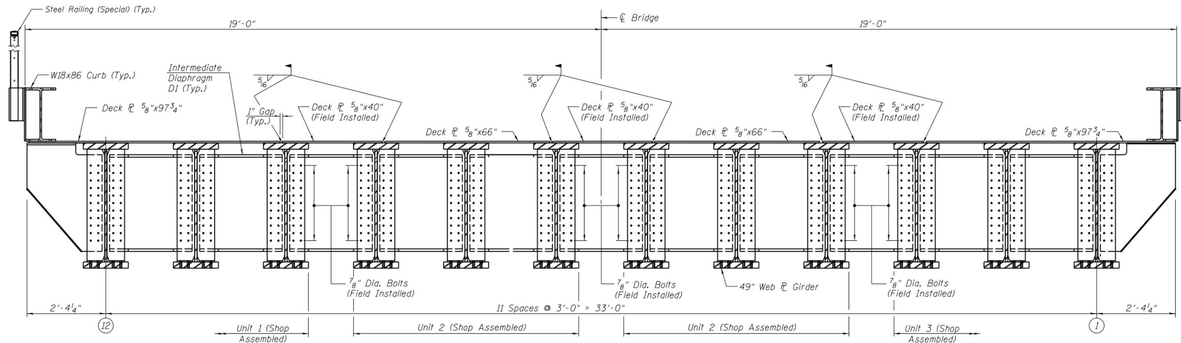
**SECTION - ASSEMBLED SPAN AT INTERIOR DIAPHRAGM**
