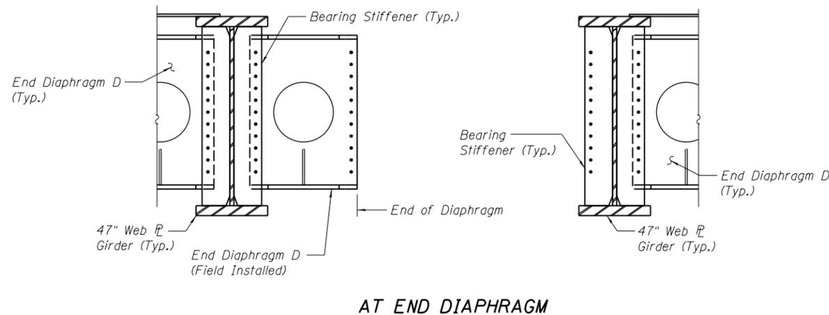
(Partial Section shown, End Diaphragm Sections are similar to Interior Diaphragm Sections except as noted above)
