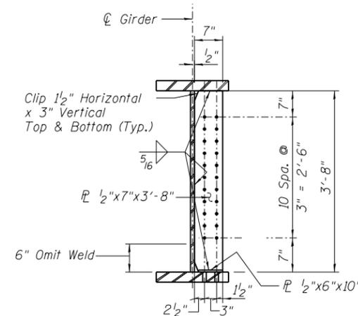
**INTERMEDIATE DIAPHRAGM CONNECTOR PLATE DI**
