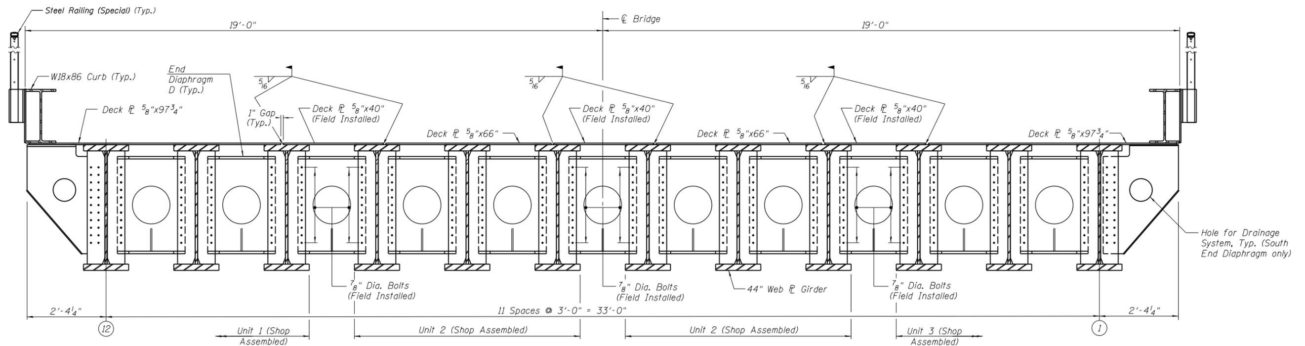
**SECTION - ASSEMBLED SPAN AT END DIAPHRAGM**
