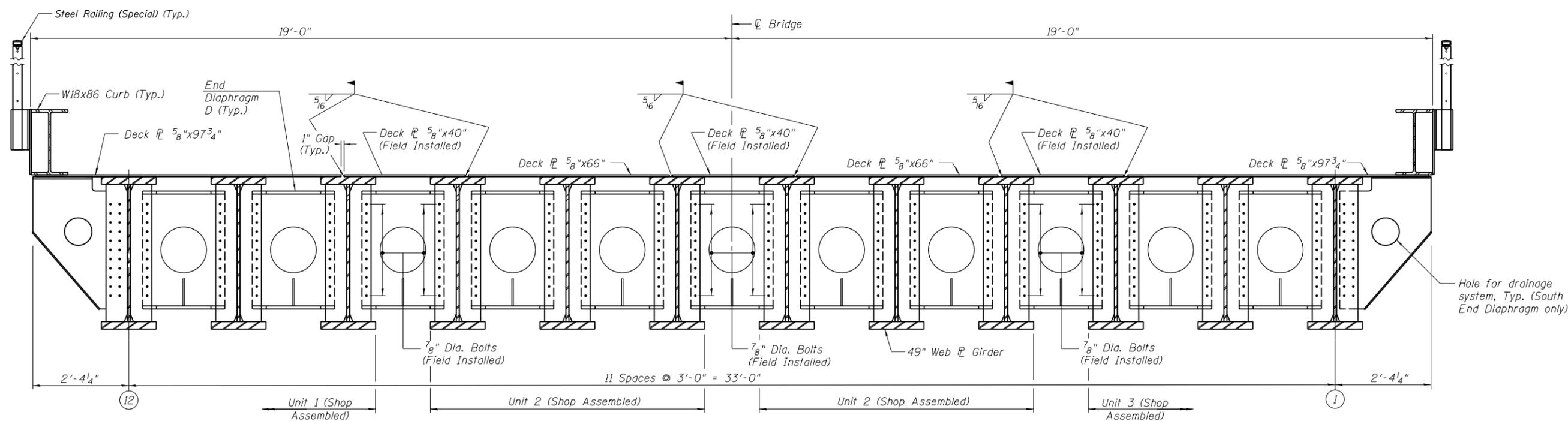
**SECTION - ASSEMBLED SPAN AT END DIAPHRAGM**
