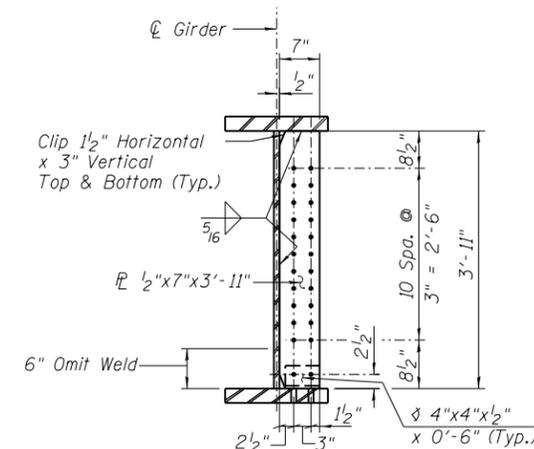
**INTERMEDIATE DIAPHRAGM CONNECTOR PLATE D1**
