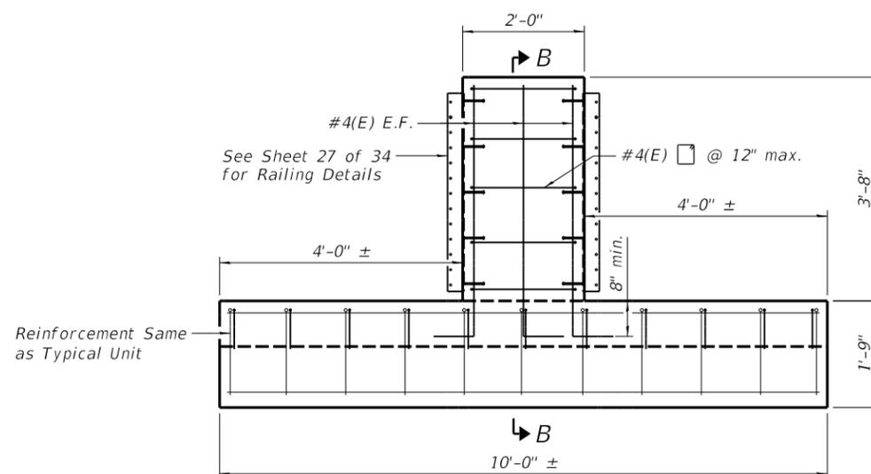
INTERMEDIATE POST UNIT ELEVATION
