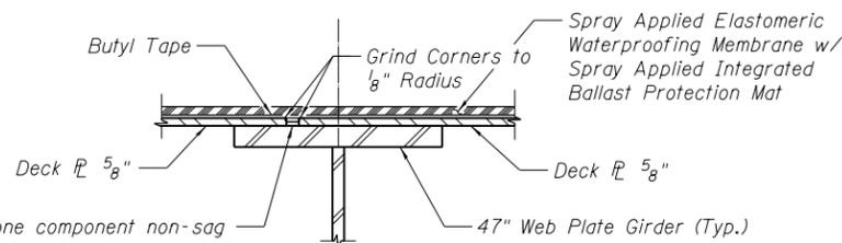
Non-staining grey one component non-sag elastomeric gun grade polyurethane sealant meeting the requirements of ASTM C-920, Type S, Grade NS, Class 25. Cost included with Membrane Waterproofing (Special)
