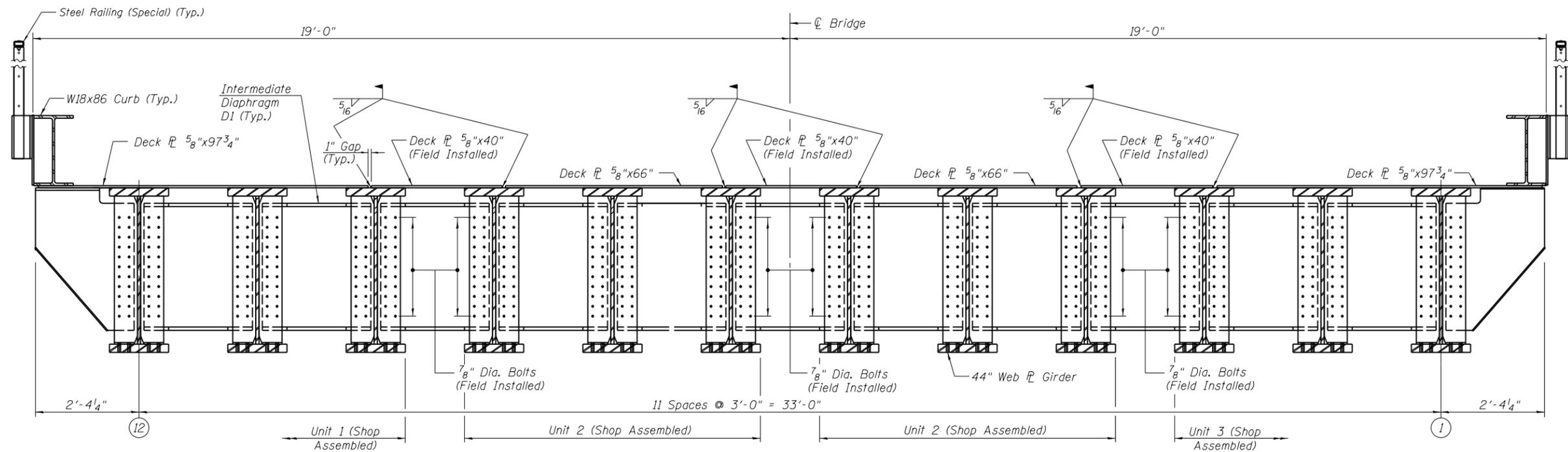
**SECTION - ASSEMBLED SPAN AT INTERIOR DIAPHRAGM**
