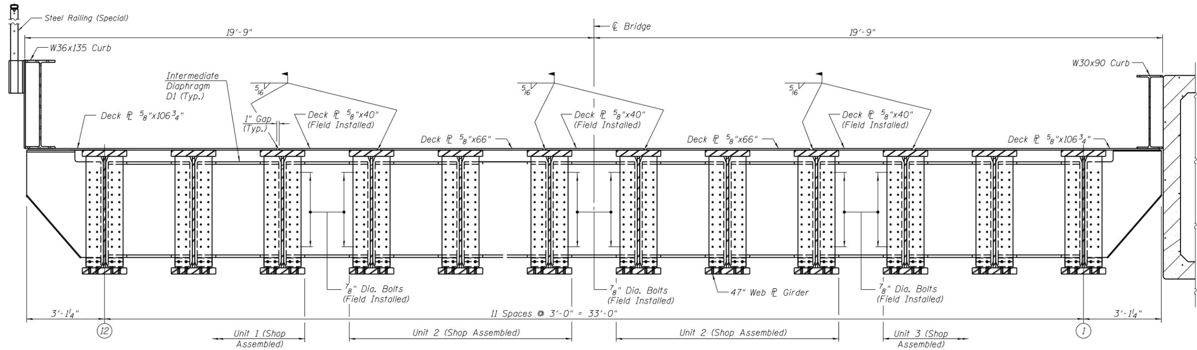
**SECTION - ASSEMBLED SPAN AT INTERIOR DIAPHRAGM**
