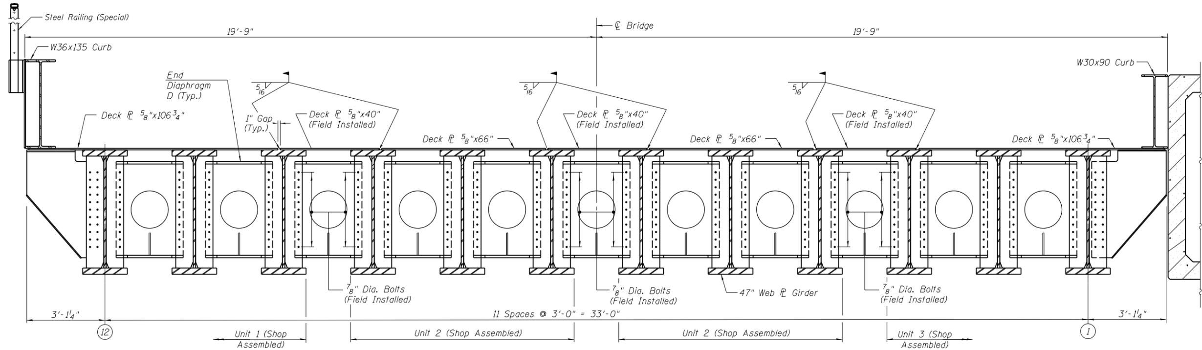
**SECTION - ASSEMBLED SPAN AT END DIAPHRAGM**
