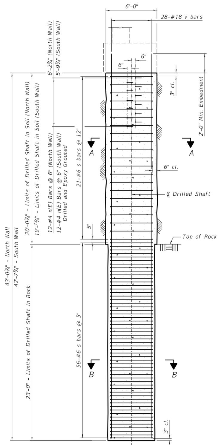
**DRILLED SHAFT ELEVATION**
