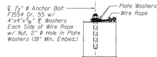
**CABLE RESTRAINT ANCHOR BOLT DETAIL**
