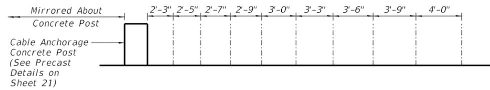
RAILING POST SPACING DETAIL
