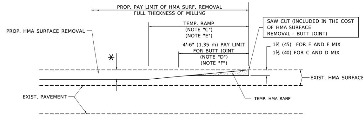
**HMA CONSTRUCTED TEMPORARY RAMP**
