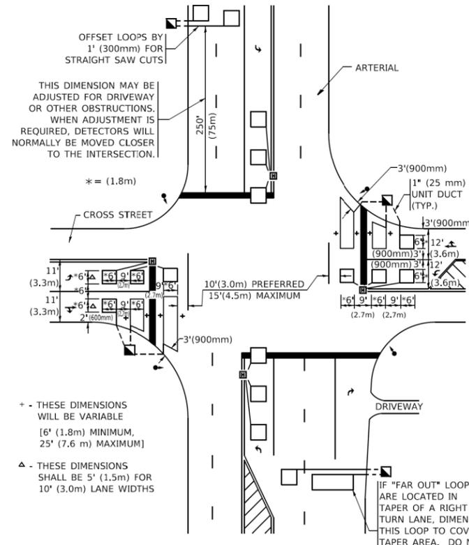
THIS DIMENSION MAY BE ADJUSTED FOR DRIVEWAY OR OTHER OBSTRUCTIONS. WHEN ADJUSTMENT IS REQUIRED, DETECTORS WILL NORMALLY BE MOVED CLOSER TO THE INTERSECTION.
