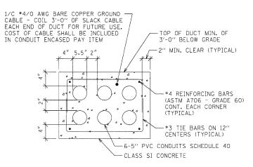
TELEPHONE/DATA DUCT BANK DETAIL NOT TO SCALE
