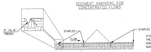
STAPLES SHALL BE PLACED WHERE THE UNITS OVERLAP AND IN THE CENTER OF THE 7' UNIT AS SHOWN ONTHE DIAGRAMS
