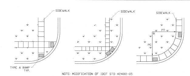
HATCHED AREAS OR DETECTABLE WARNINGS SHALL BE MANUFACTURED PRODUCTS SET IN THE POURED SIDEWALK. PROVIDE DETECTABLE WARNINGS MADE OF GLASS AND CARBON REINFORCED COMPOSITE, AS MANUFACTURED BY ADA SOLUTIONS, INC OF N. BILLERICA, MA OR EQUALLY APPROVED SUPPLIER. BOX OUTS WITH POURED COLORED CONCRETE WILL NOT BE ALLOWED. PHYSICAL CHARACTERISTICS: COMPRESSIVE STRENGTH 28,900 PSI (ATSM D695), FLEXURAL STRENGTH 29,300 PSI (ATSM D790), SLIP RESISTANCE 1.18 DRY/1.05
