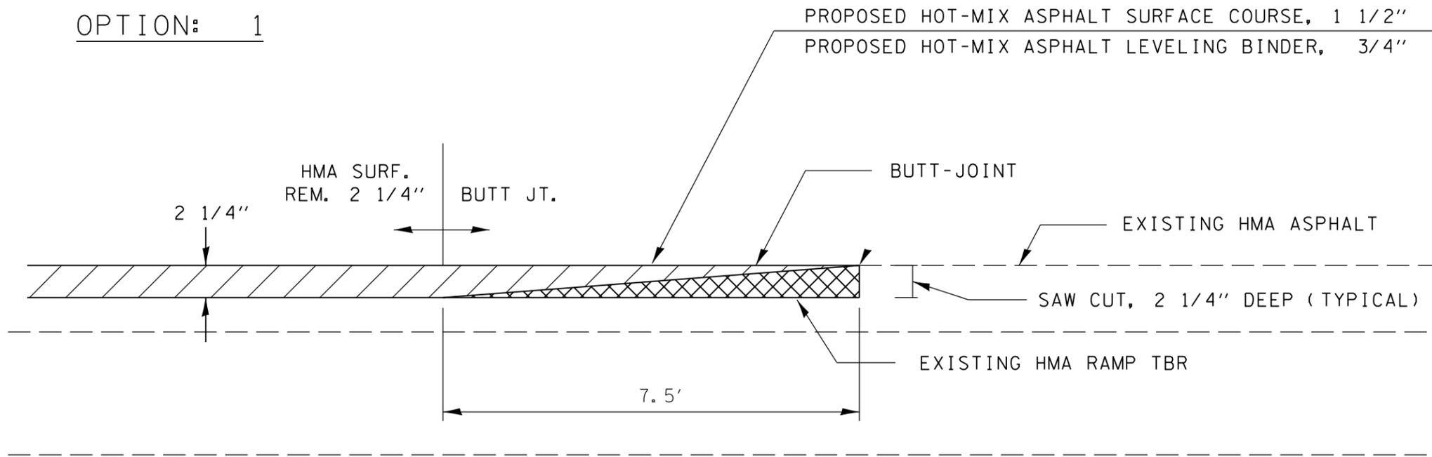
NOTE: RAMPING DOWN DURING HOT-MIX ASPHALT SURFACE REMOVAL, 2 1/4" WILL NOT BE PAID FOR AS TEMPORARY RAMP.
