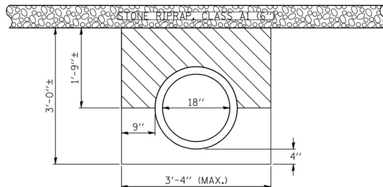
PAY LIMITS OF POROUS GRANULAR EMBANKMENT (CA-6) = 6.8 CU.YD.
