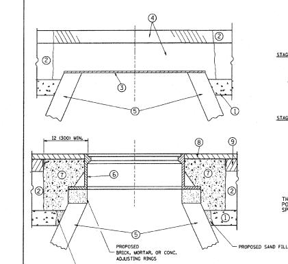
EXISTING BROKEN FRAMES AND LIDS SHALL BE REMOVED AND DISPOSED OF BY THE CONTRACTOR AND SHALL BE REPLACED AS DIRECTED BY THE ENGINEER. REPLACEMENT FRAMES AND LIDS WILL BE PAID FOR IN ACCORDANCE WITH ARTICLE 109.04 OF THE STANDARD SPECIFICATIONS UNLESS A SEPARATE PAY ITEM HAS BEEN PROVIDED.
