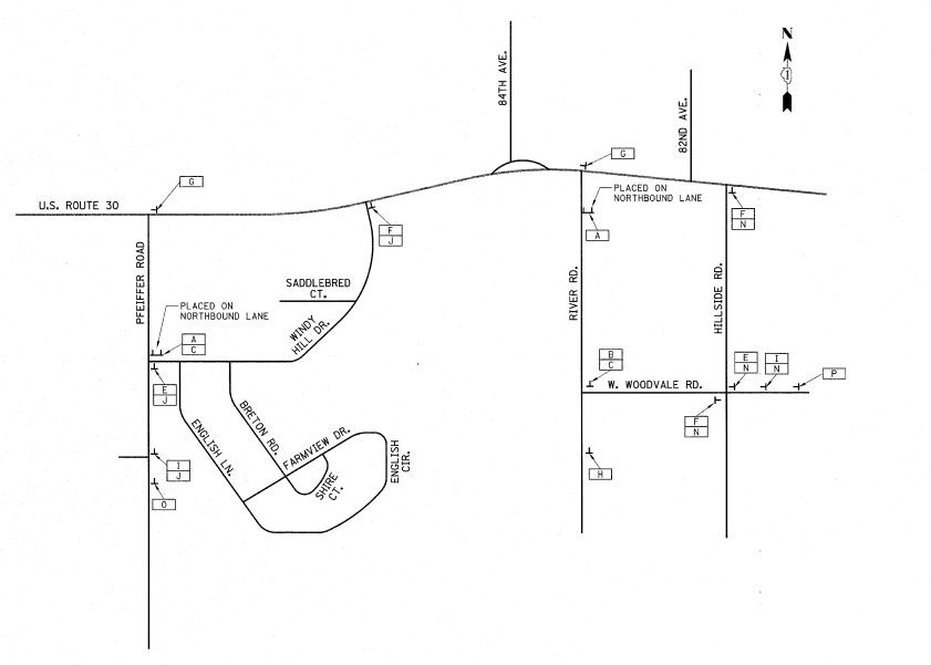
R11-2 48" × 30"  $\bigcirc$ CLOSED ROAD CLOSED TO THRU TRAFFIC  $^{\otimes}$ 60" × 30" MR-10(R) MR-10(L) 48" × 18" M4-9(R) (E) 30" × 24" M4-9(L) 30" × 24" F END M4-8A (G) 24" x 18" DETOUR ROAD W20-3 48" x 48" CLOSED AHEAD W20-2 48" × 48" 1
