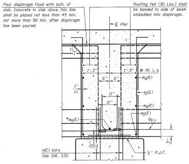
SECTION B-B Dimensions along  $\@model{\ell}$  of beam, except as shown. \* Tightly fasten the #8 bars together with No. 9 wire ties.
