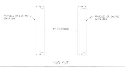
WHEN PROPOSED SEWER (OR WATER) IS LOCATED LESS THAN 10 FEET FROM EXISTING WATER (OR SEWER), DETAILS BELOW SHALL APPLY. SEE ARTICLE 41-2.01B (2)
