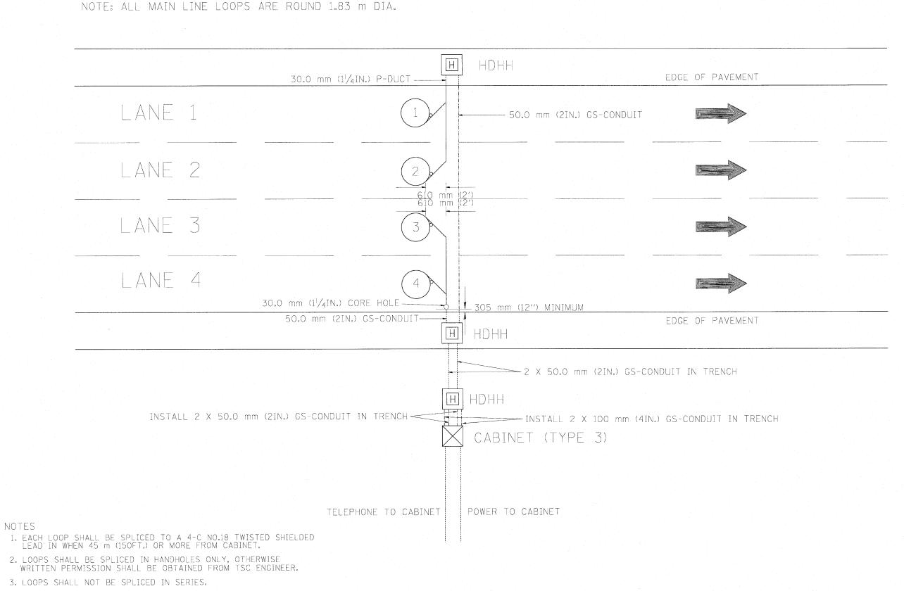
4. EACH LOOP LEAD IN SHALL BE IDENTIFIED AND PERMANENTLY COLOR CODED IN THE COREHOLE, HANDHOLE & CABINETS THRU WHICH THEY ENTER OR PASS AND TAGGED WITH THE CORRECT NOMENCLATURES.
