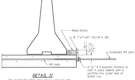
The 1"x7"x10" Plate shall not be removed until Stage II Construction forms and all reinforcement bars are in place and the concrete is ready to be placed.
