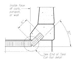
AT CURB, PARAPET, OR WALL (Showing seal)
