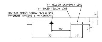
TYPICAL APPLICATION FOR BI-DIRECTIONAL TURN LANE WITH RAISED REFLECTIVE PAVEMENT MARKERS
