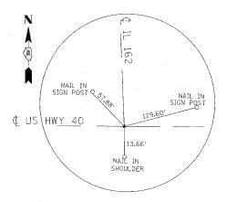
NAIL IN PAVEMENT POT STA. 719+45.59 (IL 162) POT STA. 100+00.00 (US HWY 40) N 746,968.18 E 2,389,049.95
