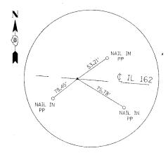
NAIL IN PAVEMENT PC STA. 705+01.65 N 747,793.10 E 2,387,937.97
