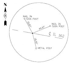
NAIL IN PAVEMENT PC STA. 717+60.23 N 747,137.52 E 2,388,995.13
