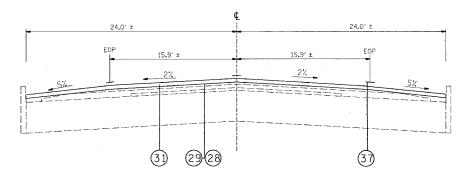
MILLING PROCEDURES: MILL  $1\frac{1}{2}$ " OF SURFACE USING THE CENTERLINE AS THE CONTROL POINT. MILL FROM THE CENTERLINE TO THE EDGE OF PAVEMENT AT A SLOPE OF 2%. THEN MILL 1/2" AT A RATE OF 5% FROM THE EDGE OF PAVEMENT TO THE CURB. THIS WORK WILL BE PAID FOR AS (BITUMINOUS SURFACE REMOVAL  $1\frac{1}{2}$ ").
