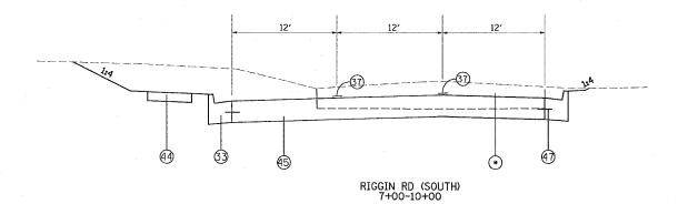
• EXISTING RIGGIN RD (SOUTH) CONSISTS OF PCC PAVEMENT - UNKNOWN DEPTH (TO BE REMOVED)
