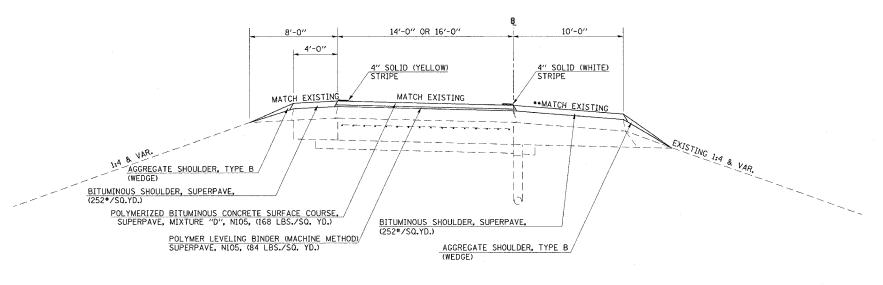
•• FOR SECTIONS ON LOW SIDE OF SUPERELEVATION: SLOPE SHOULDER SAME AS PAVEMENT, BUT NOT LESS THAN 1/2"/FT.
