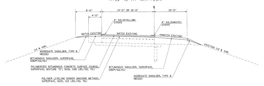
\*\* FOR SECTIONS ON LOW SIDE OF SUPERELEVATION: SLOPE SHOULDER SAME AS PAVEMENT, BUT NOT LESS THAN  $\frac{1}{2}^{\prime\prime}/\text{FT.}$
