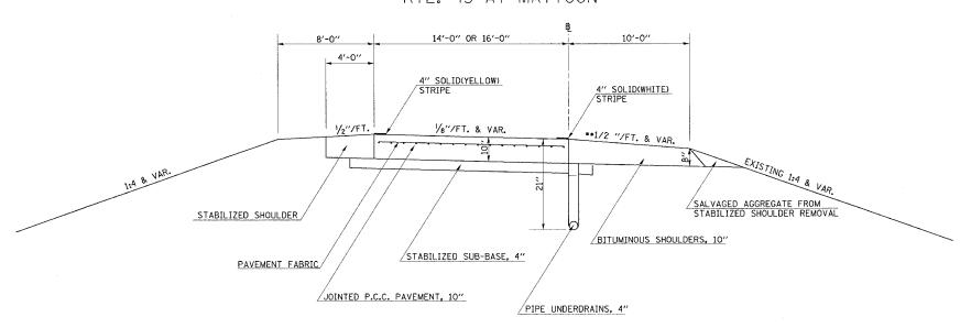
\*\* FOR SECTIONS ON LOW SIDE OF SUPERELEVATION: SLOPE SHOULDER SAME AS PAVEMENT, BUT NOT LESS THAN 1/.2 "/FT.
