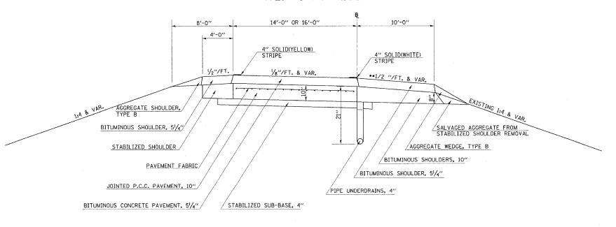
\*\* FOR SECTIONS ON LOW SIDE OF SUPERELEVATION: SLOPE SHOULDER SAME AS PAVEMENT, BUT NOT LESS THAN 1/.2 "/FT.
