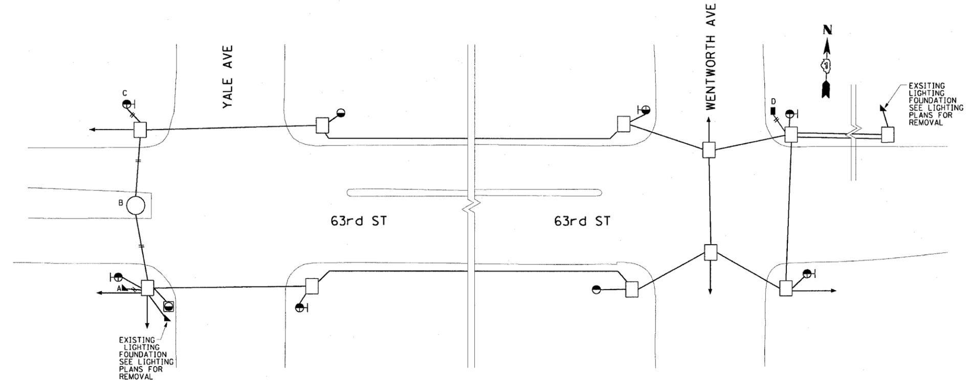
**FOUNDATION AND CONDUIT REMOVAL PLAN**
