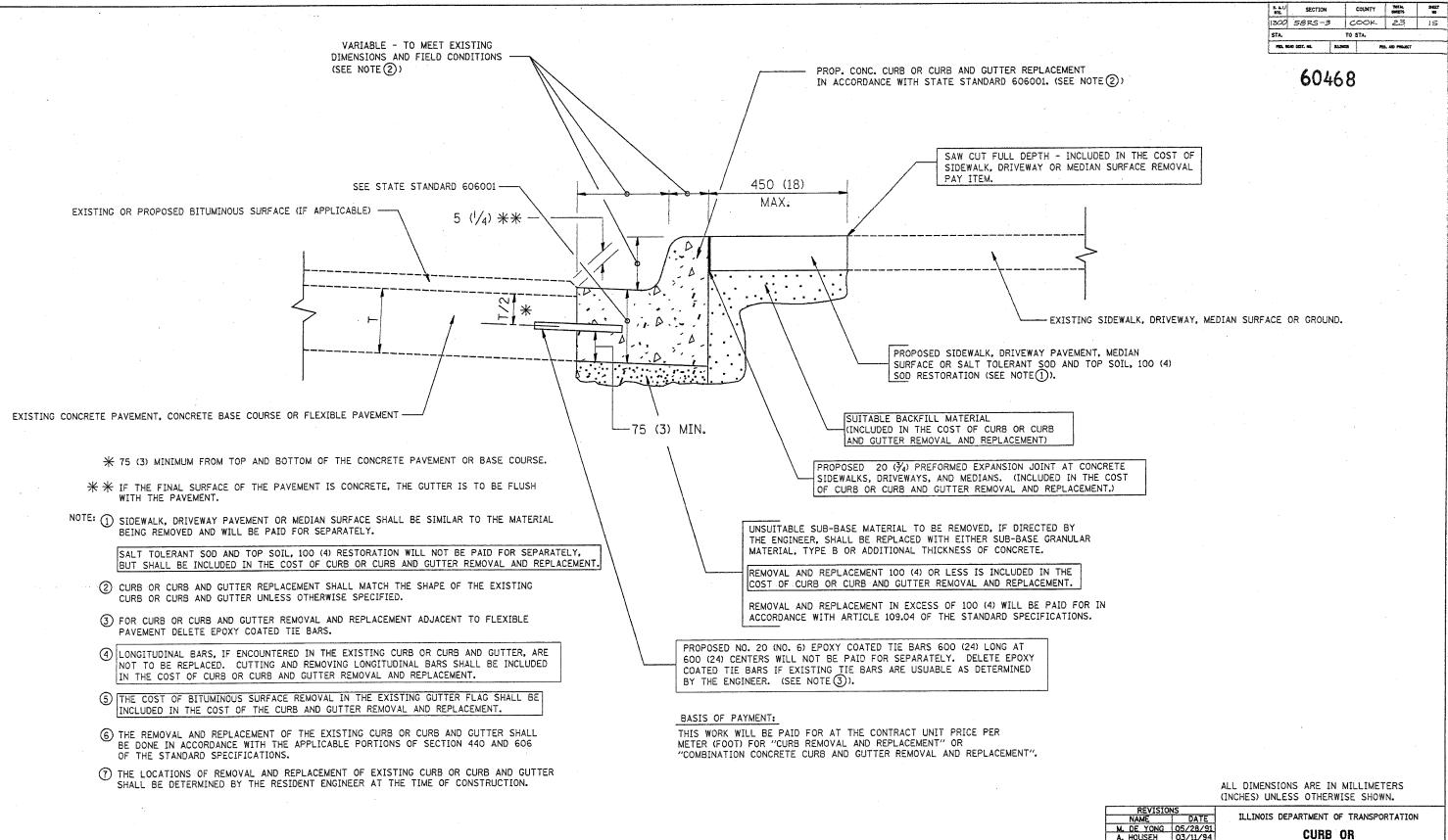
**CURB OR CURB AND GUTTER REMOVAL AND REPLACEMENT**
