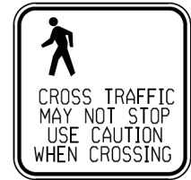
CROSS TRAFFIC MAY NOT STOP USE CAUTION WHEN CROSSING SIGN (12" x 12") PEDESTRIAN SYMBOL HEIGHT - 4" (IN) LETTERS - 1" C LEGEND - BLACK BACKGROUND - YELLOW
