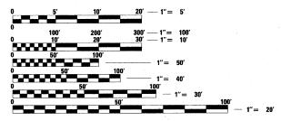
ENGINEERING SCALES, REDUCED SIZED PLANS WILL NOT CONFORM TO STANDARD SCALES. IN MAKING MEASUREMENTS ON REDUCED PLANS, THE ABOVE SCALES MAY BE USED.
