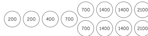
SAND MODULE IMPACT ATTENUATOR LAYOUT
