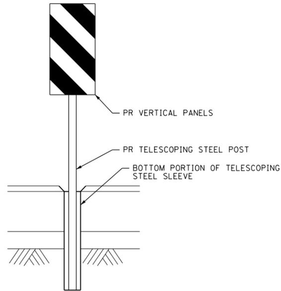
NOTE: FOR INSTALLATION OF VERTICAL PANELS IN AREAS OF CROSSOVER PAVEMENT, 3" Ø HOLES WILL BE CORED THROUGH PAVEMENT FOR PLACEMENT. TELESCOPING STEEL POLES WILL BE PLACED 1" BELOW SURFACE AS SHOWN, AND WORK SHALL BE DONE TO THE SATISFACTION OF THE ENGINEER. WHEN OPENING CROSSOVER, PANELS WILL BE REMOVED AND HOLES WILL BE LEFT IN PLACE. COST OF PANELS, POSTS, SLEEVES, TYPE III BARRICADES, SIGNS, AND CORING SHALL BE INCLUDED IN TRAFFIC CONTROL AND PROTECTION (SPECIAL).
