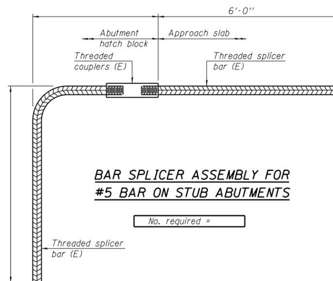
**BAR SPLICER ASSEMBLY FOR #5 BAR ON STUB ABUTMENTS**
