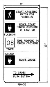
THE CONTRACTOR SHALL SUPPLY AND MOUNT ONE SIGN AT EACH EXISTING PEDESTRIAN PUSH-BUTTON AND THIS SHALL BE INCLUDED IN THE COST OF PEDESTRIAN SIGNAL HEAD PAY ITEM.
