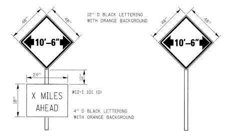
A TOTAL OF FOUR POST MOUNTED SIGNS ARE REQUIRED:
