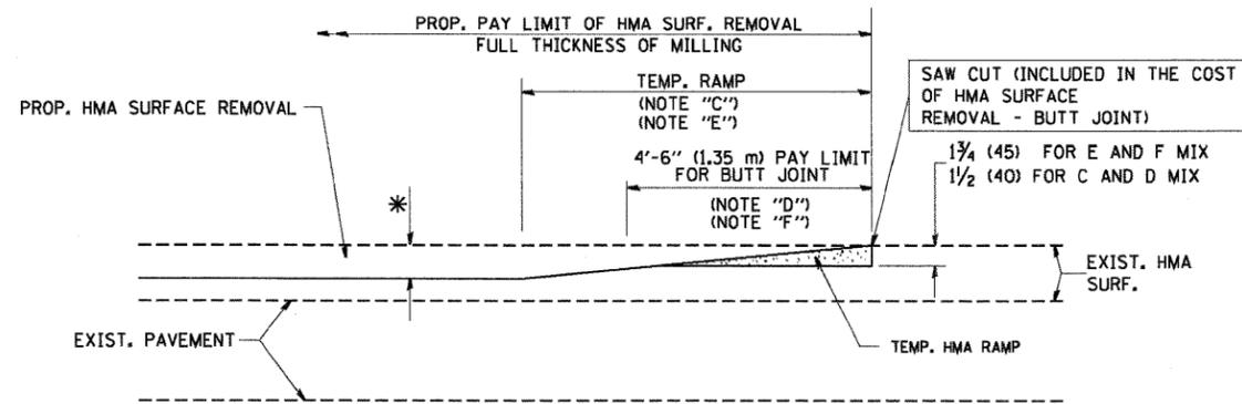
HMA CONSTRUCTED TEMPORARY RAMP
