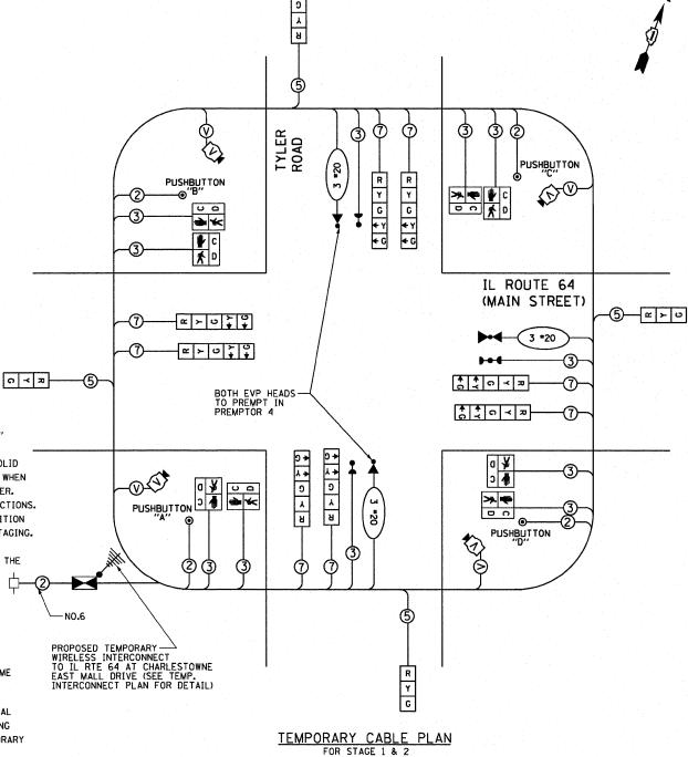
PUSHBUTTON "A" SHALL PLACE A CALL IN PHASES 2 AND 4 PUSHBUTTON "B" SHALL PLACE A CALL IN PHASES 4 AND 6 PUSHBUTTON "C" SHALL PLACE A CALL IN PHASES 6 AND 8 PUSHBUTTON" D" SHALL PLACE A CALL IN PHASES 2 AND 8
