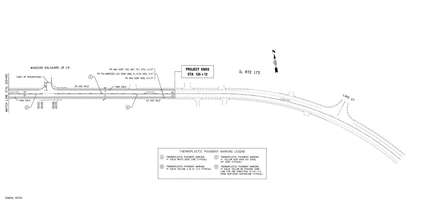
1) ALL RAISED REFLECTIVE PAVEMENT MARKERS SHALL BE PLACED IN ACCORDANCE WITH DISTRICT ONE "TYPICAL APPLICATIONS RAISED REFLECTIVE PAVEMENT MARKERS (SNOW-PLOW RESISTANT) (TC-11)" STANDARD DETAIL.
