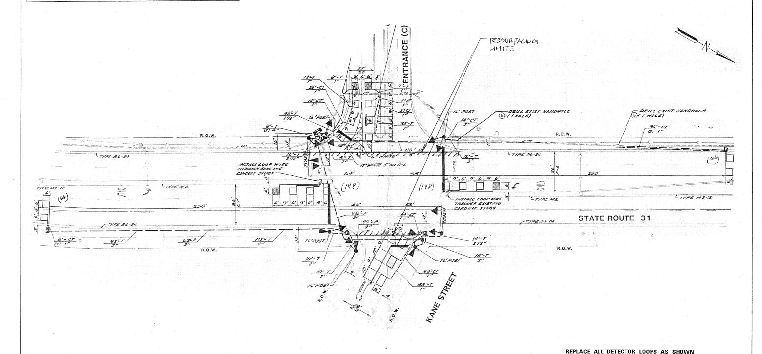
THIS PLAN IS FOR THE SOLE PURPOSE OF **DETECTOR LOOP REPLACEMENTS ONLY**
