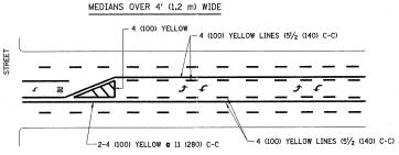
A MINIMUM OF TWO PAIRS OF TURN ARROWS SHALL BE USED, WHITE IN COLOR. ADDITIONAL PAIRS SHALL BE PLACED AT 200' (60 m) TO 300' (90 m) INTERVALS.
