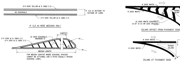
DIAGONAL LINE SPACING: 50' (15 m) C-C (LESS THAN 30MPH (50 km/h))
