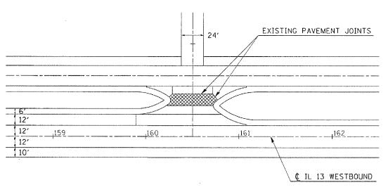
PCC SURFACE REMOVAL, BUTT JOINT
