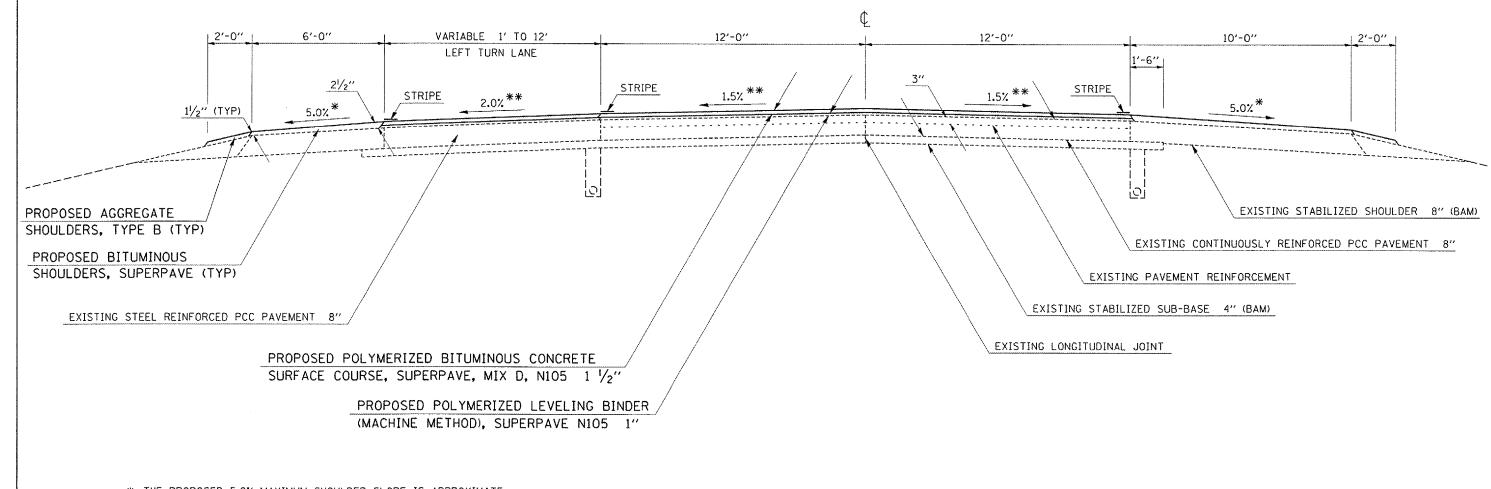
\* THE PROPOSED 5.0% MAXIMUM SHOULDER SLOPE IS APPROXIMATE. THE SLOPE SHALL BE ACCOMPLISED BY TAPERING THE SHOULDER MIX FROM  $2\frac{1}{2}$ " AT THE EDGE OF PAVEMENT TO  $1\frac{1}{2}$ " MINIMUM AT THE EDGE OF SHOULDER.
