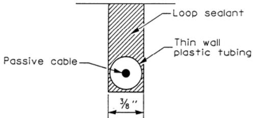
The passive cable can be put in a thin wall plastic tube for additional protection.
