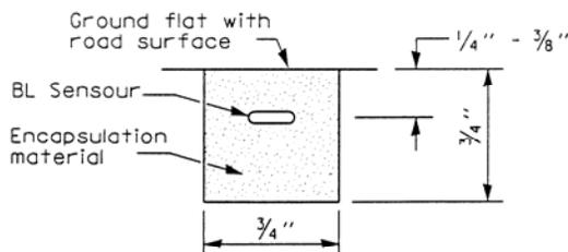
Typical cross section of a BL Sensor installation.
